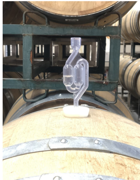
As Chardonnay ferments in barrel we use a water lock; a one way valve to let gas escape but without letting air in
